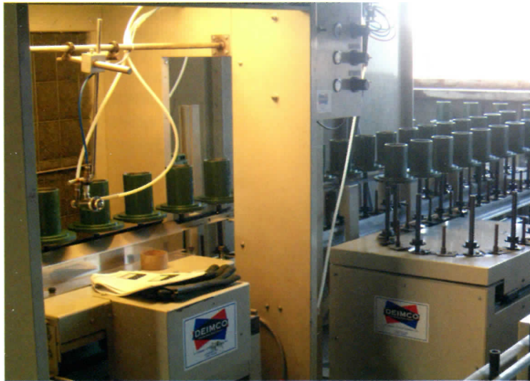
Above: Custom finishing cell designed for casing and line coupling manufacturers. Capable of handling casings up to 14-3/8" outer diameter and up to 70 pounds each. (Liquid cell)
