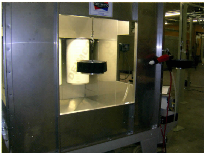
Above: Motor stator manually coated as it rotates through MD1600 booth
