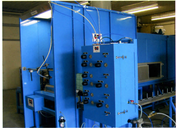
Above: Large part liquid chain-on-edge cell for finishing electrical components.
